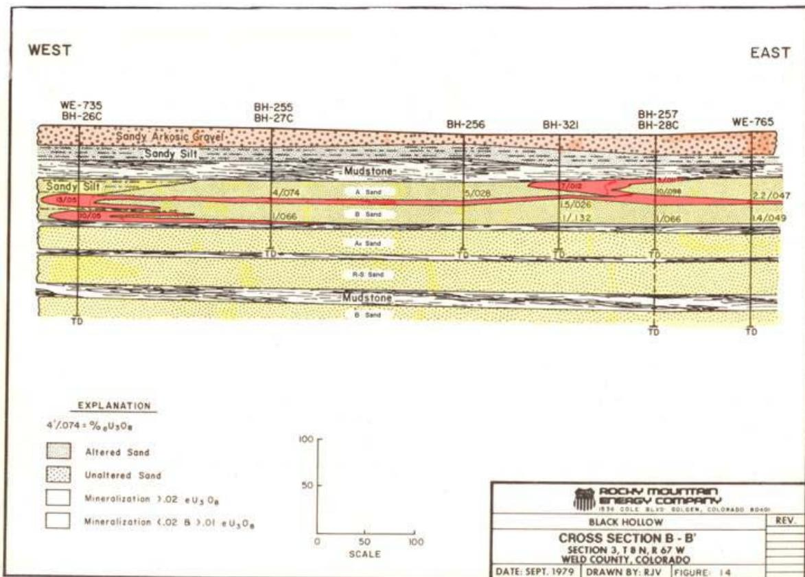
Figure 10 Cross-section of mineralized Fox Hill sands in the southern portion of the Centennial Project Source: RME files
