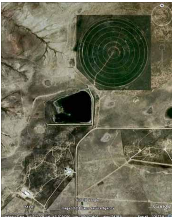
Figure 20: Aerial photo of the Highland Ranch project, showing ISL well complexes (lower left), a purge storage reservoir (center), and a pivot irrigation field (top) where in-situ leach leaching solutions are disposed of through irrigation after treatment. The U.S. Fish & Wildlife Service has documented the bioaccumulation of radioactive selenium in the food chain within in-situ leach pivot irrigation fields. Source: Ramirez and Rogers, Selenium in a Wyoming Grassland Community Receiving Wastewater From an In Situ Uranium Mine .
