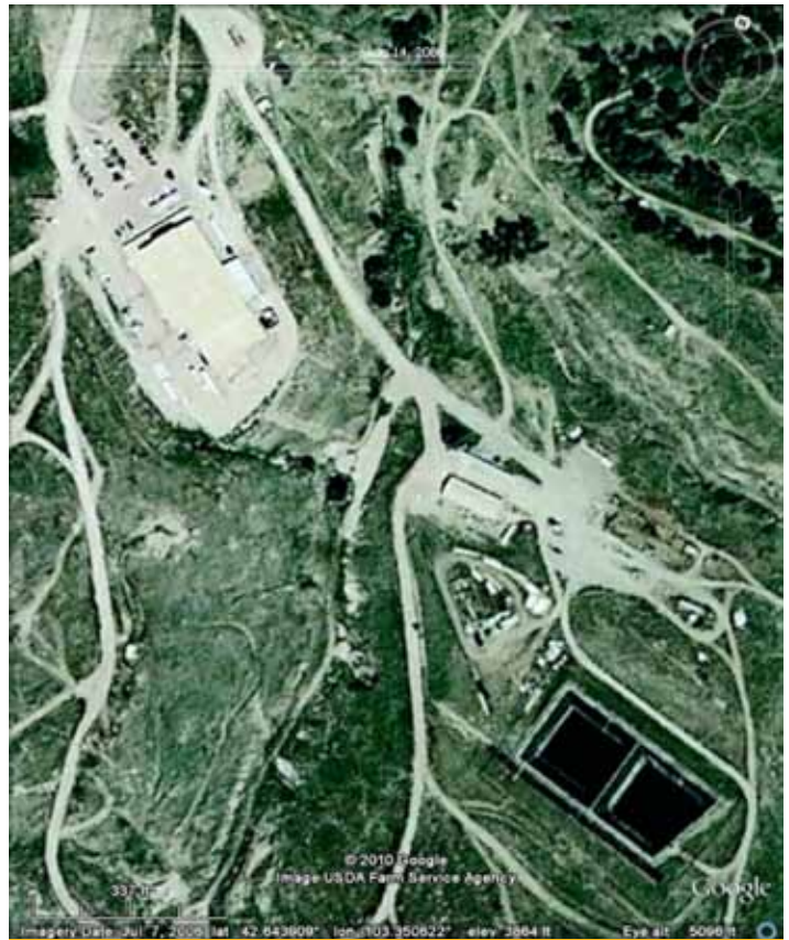
Figure 16: Aerial photo of the of processing plant (upper left) and two evaporation ponds (lower right) at Cameco’s Crow Butte uranium in-situ leach facility in Dawes County, Nebraska. Source: Google Earth.
