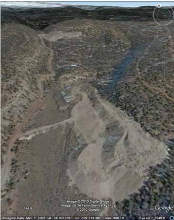
Figure 12: Aerial photograph of the Pandora uranium mine in San Juan County, Utah, owned by Denison Mines. Pandora is accessed by spiral tunnels, or declines, from the surface and is connected underground with the adjacent Beaver mine, 1.5 kilometers northwest of Pandora and not visible here. Pandora, a mature conventional uranium mine with extensive underground workings, produced 52,000 tons of ore in 2008. Source: Google Earth.
