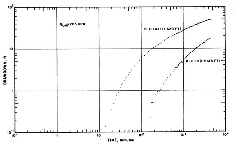
Figure 15: Logarithmic Graphs of Drawdown for B-II Observation Well Group, Lakota Aquifer Test
