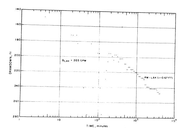
Figure 7: Semilogarithmic Graph of Drawdown for Pumped Well, Lakota Aquifer Test
