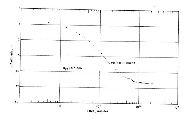
Figure 26: Semilogarithmic Graph of Drawdown for the Pumped Well,
