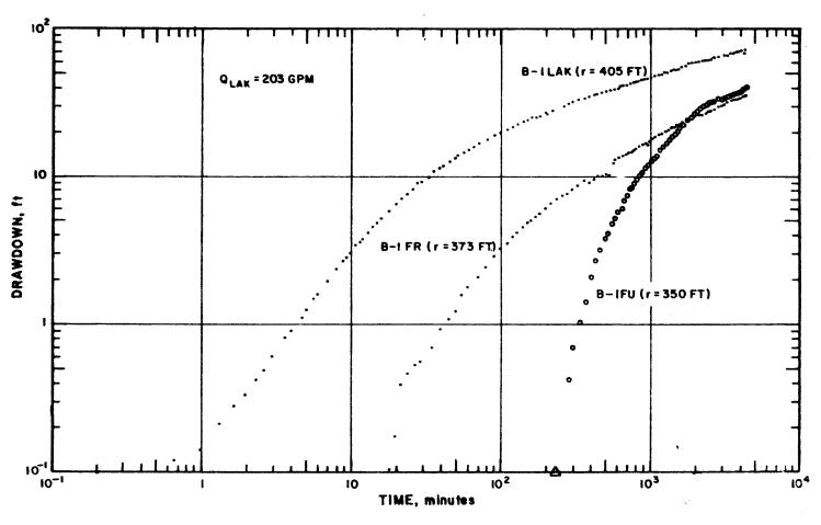
Figure 14: Logarithmic Graphs of Drawdown for B-1 Observation Well Group, Lakota Aquifer Test
