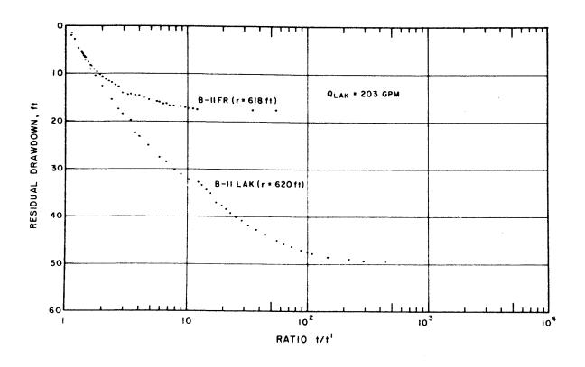
Figure 23: Recovery Graphs for B-II Observation Well Group, Lakota Aquifer Test
