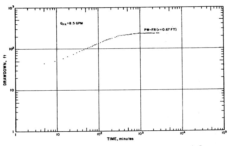
Figure 30: Logarithmic Graph of Drawdown for Pumped Well, Fall River Aquifer Test
