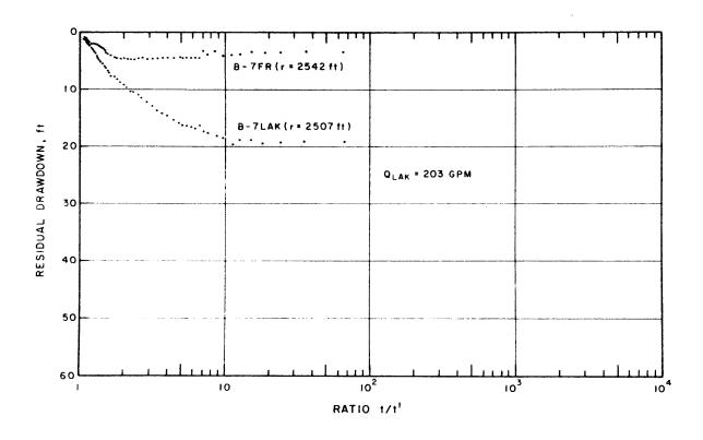
Figure 25: Recovery Graphs for B-7 Observation Well Group, Lakota Aquifer Test
