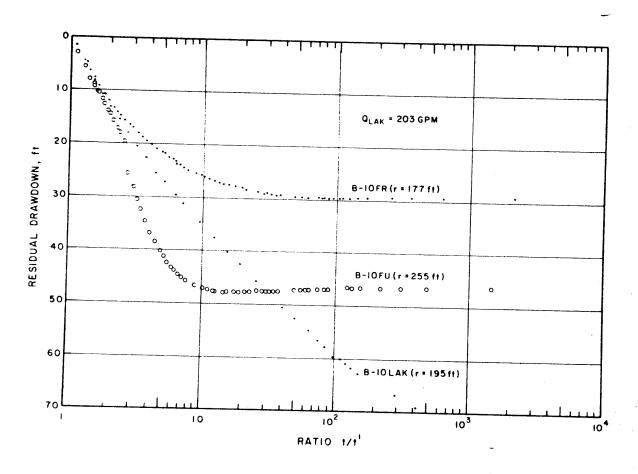
Figure 21: Recovery Graphs for B-10 Observation Well Group, Lakota Aquifer Test
