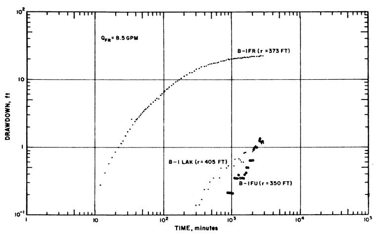
Figure 32: Logarithmic Graphs of Drawdown for B-1 Observation Well Group, Fall River Aquifer Test
