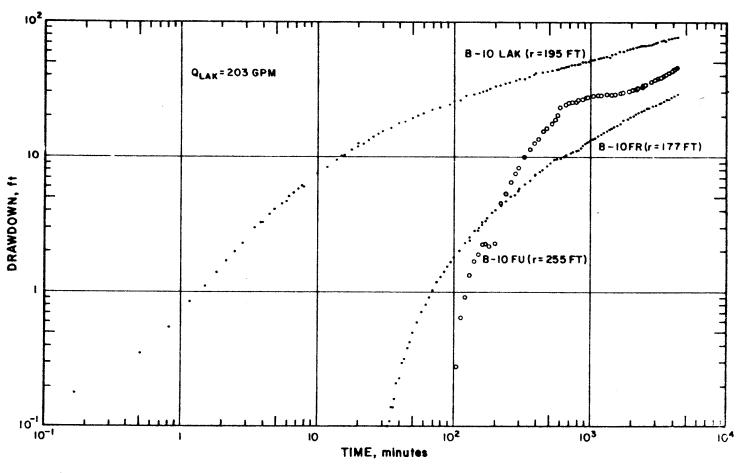
Figure 13: Logarithmic Graphs of Drawdown for B-10 Observation Well Group, Lakota Aquifer Test
