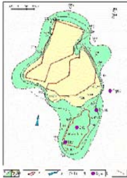
FIG. 33. Scheme of spreading sulphate-ion for period 1988-1999 on ore unit 1k of Kanzhugan deposit Legend: 1) isopleths of sulphate-ion concentration (g/l) at the state of 1988 (a) and 1999 (b); 2) contour of ore unit; 3) the direction of groundwater flow; 4) a monitoring well and its number; 5) wells drilled under the EIA project; 6) front of oxidation.
